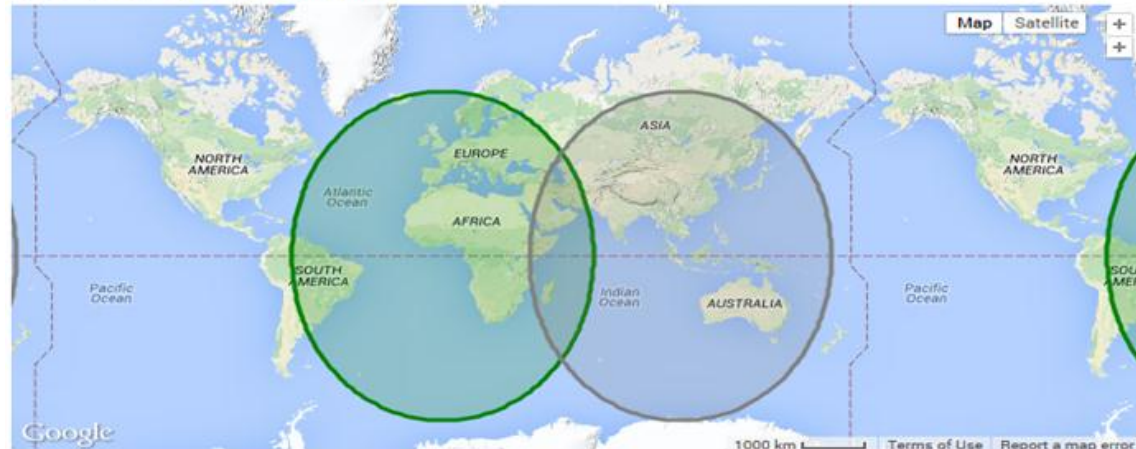
The following interactive map shows the nominal footprints of these satellites (Assuming a zenith angle of 75°) : Show / Hide all footprints
