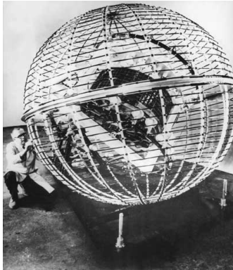
Pre-launch tests of meteorological satellite TIROS (1960)
